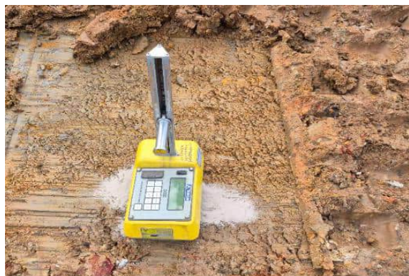
Photo 9: Field density/moisture test
