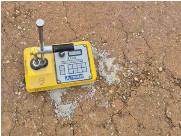
Photo 9: Field density/moisture test
