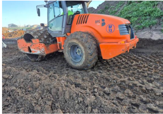
Photograph 6: Pad foot roller used during fill construction
