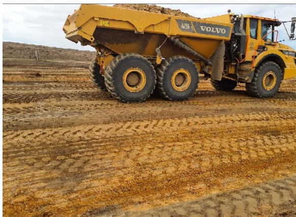
Photograph 3: Subgrade assessed with loaded dump truck
