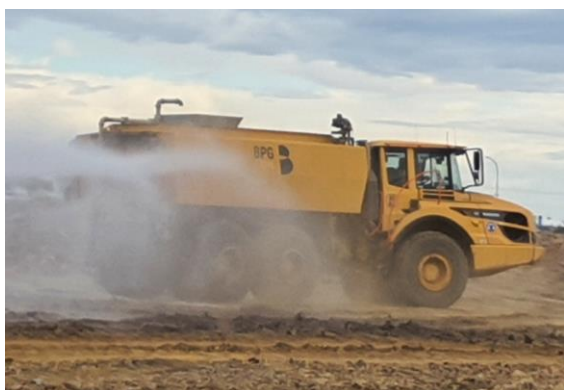
Photograph 7: Water cart during fill construction
