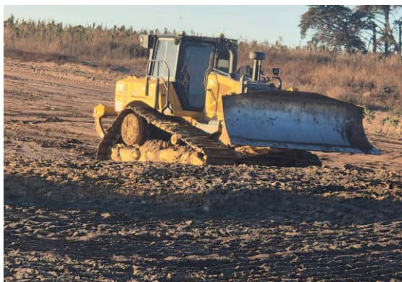
Photograph 5: Dozer used during fill construction
