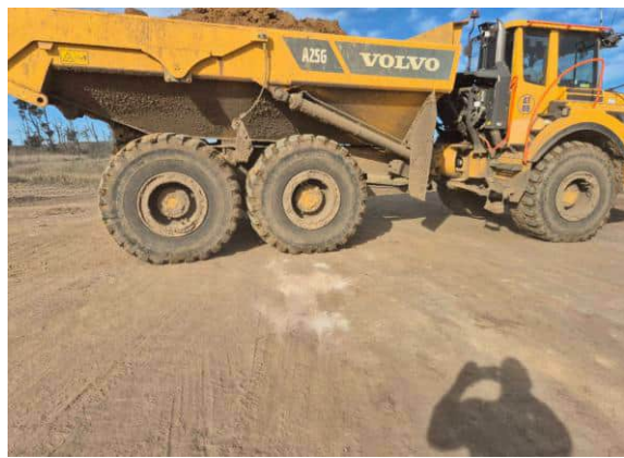
Photograph 4: Subgrade assessment using loaded dump truck
