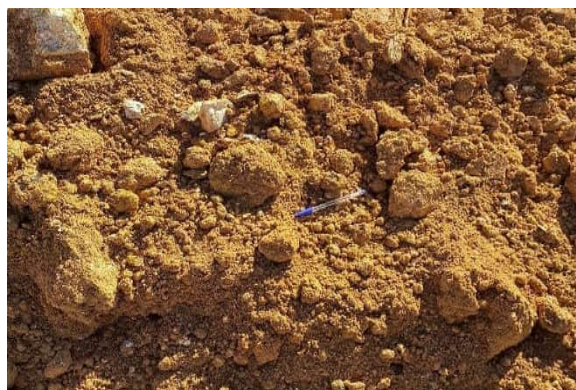
Photograph 1: sandy clay imported material used on site
