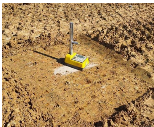
Photo 10: Field density/moisture test
