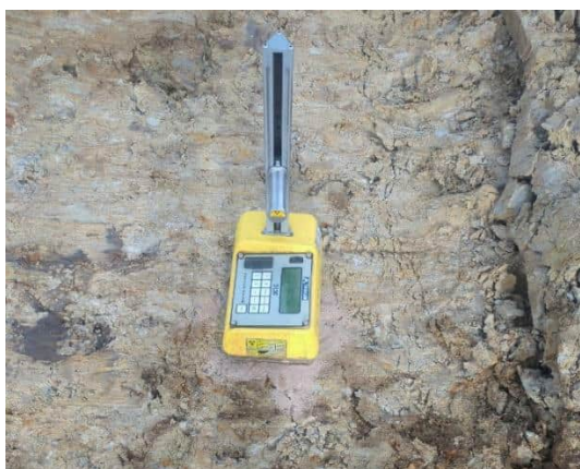
Photo 9: Field density/moisture test
