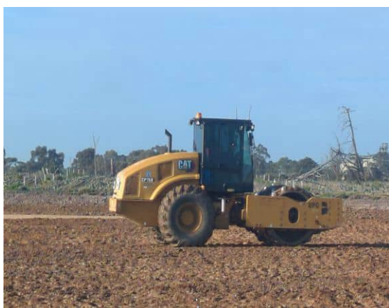
Photograph 7: Compactor used during fill construction
