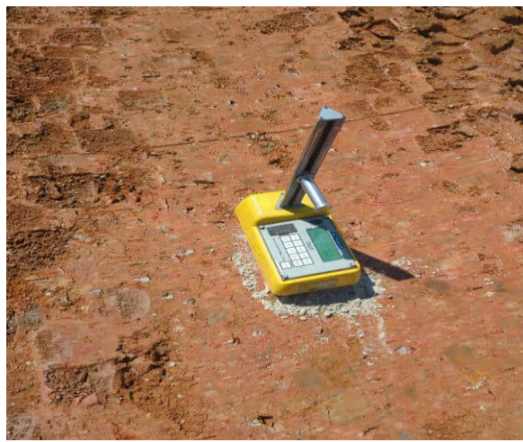
Photo 10: Field density/moisture test
