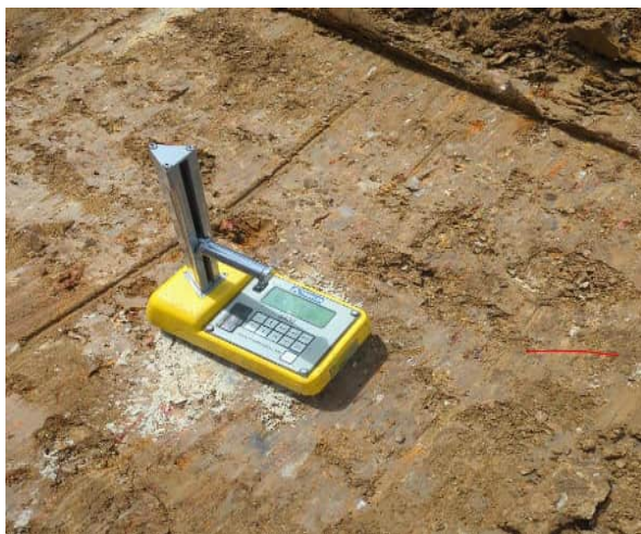
Photo 9: Field density/moisture test
